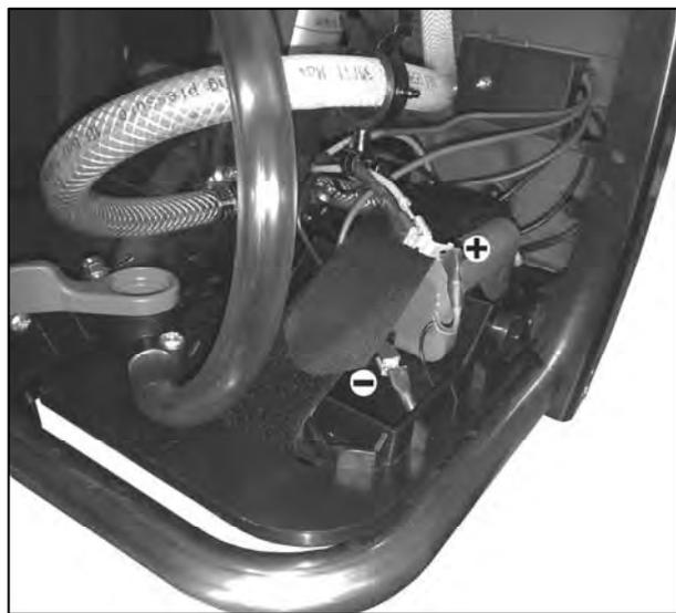
**Positive terminal:** Connect the red wire-plug of the battery on the cable connector with the red cable. This cable connector is secured with a clamp on the upper hose.
