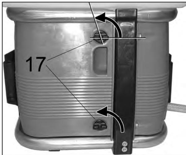
To open the protective casing, rotate both locking buttons (17) approximately 100° anti-clockwise. Open the protective casing.
